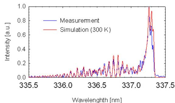
Figure 1. Measurement and simulation for the 0-0 transition of the 2<sup>nd</sup> positive system of nitrogen in the OES of the helium DBD with ultrasonic irradiation. The best fit was found for a rotational temperature of 300 K. The measured spectral resolution (FWHM) is 20 pm.
