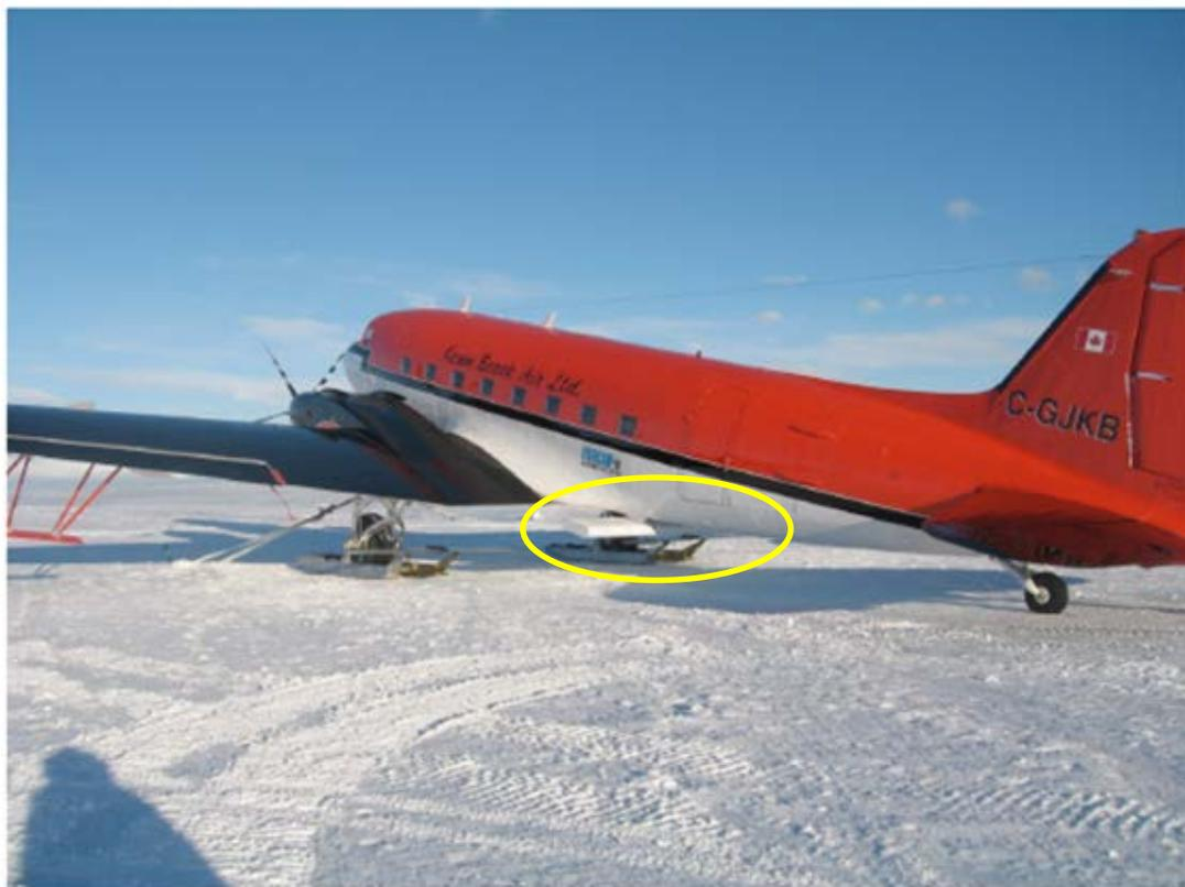
Figure 7: Basler DC-3 with the POLARIS antenna mounted under the fuselage
