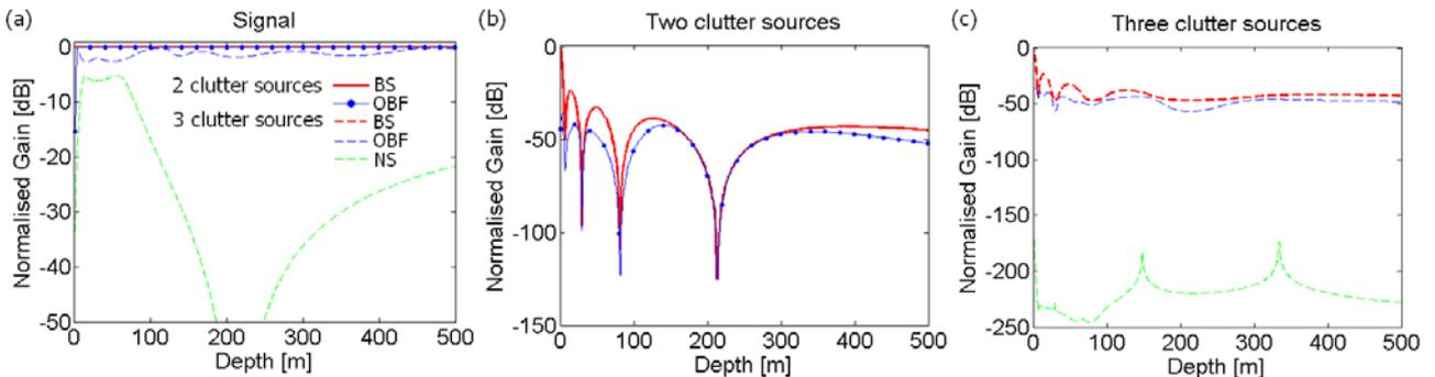
Figure 6: Result of sensitivity analysis of the normalized signal gain (a) and the normalized summed clutter gain, assuming beam-steering, null-steering and the optimum beamformer, for 2 (b) and 3 (c) clutter sources.
