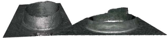
Fig.2. 3D reconstruction of burr scanned by infinite focus 3D microscope.
