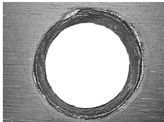
Fig.7. Hole entry defect.
