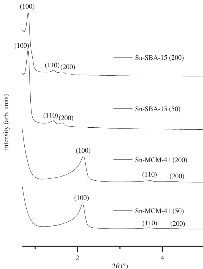
Figure 3. Diffraction pattern of the mesoporous stannosilicates.
