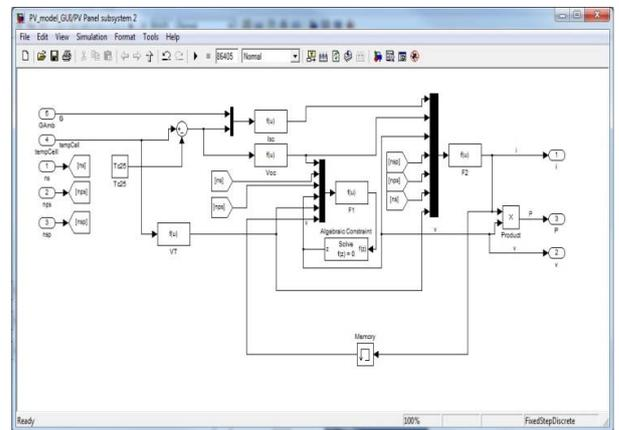
Fig. 2. PV string model implemented in Simulink
