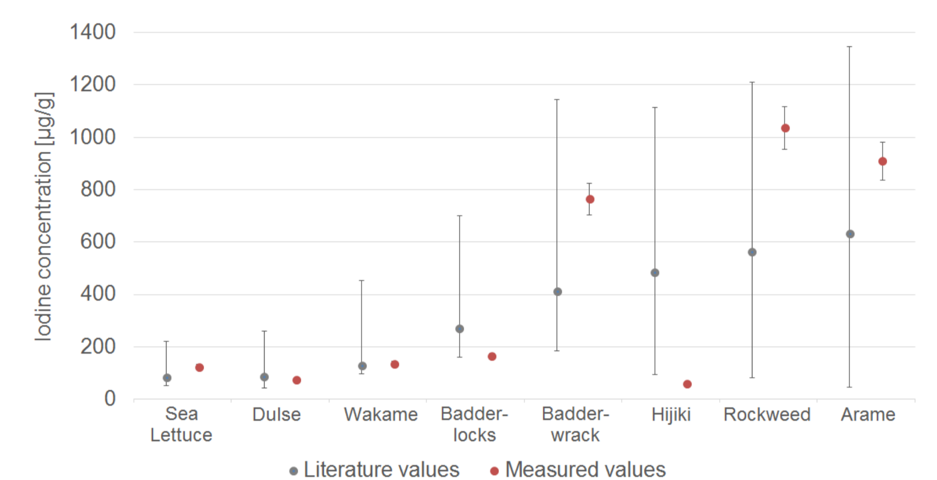
Figure 3. Determination of the total iodine content in seaweed samples compared with literature values (dry weight). Measured values are shown with error lines for 2 SD corresponding to a 95% confidence interval. Literature values are shown with error lines for the total range of measured values. LOD method = 0.03 µg/g.
