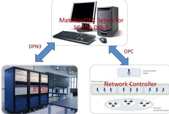
Figure 2 Simulation platform for active distribution network controller
