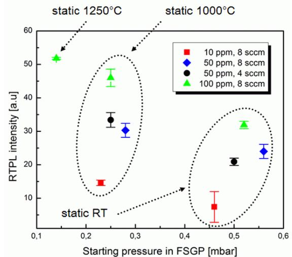
**Fig. 4** Room temperature PL peak intensity as a function of starting pressure in sublimation epitaxy for samples grown from differently doped sources. Static vacuum modification used is indicated.
