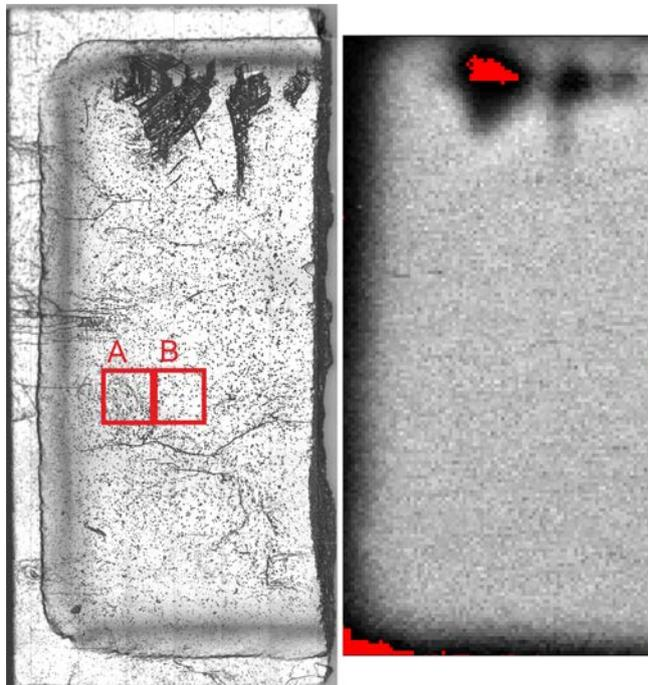
**Fig. 1** Microscope map of sample ELS375 after defect-selective etching with the corresponding RTPL map (legend shows PL intensity in arbitrary units). The dark areas at the upper edge of the samples are inclusions of 3C-SiC.
