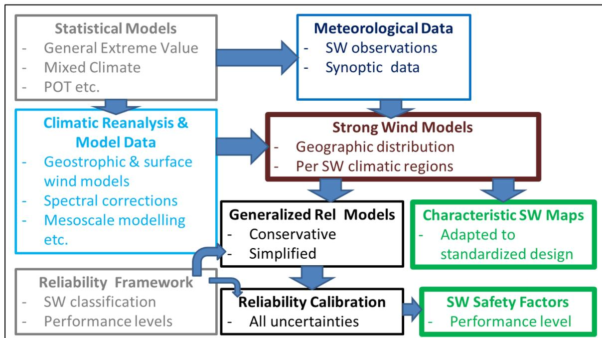
Figure 7. Summary of an optimal approach for the estimation of design wind speeds from climate data.
