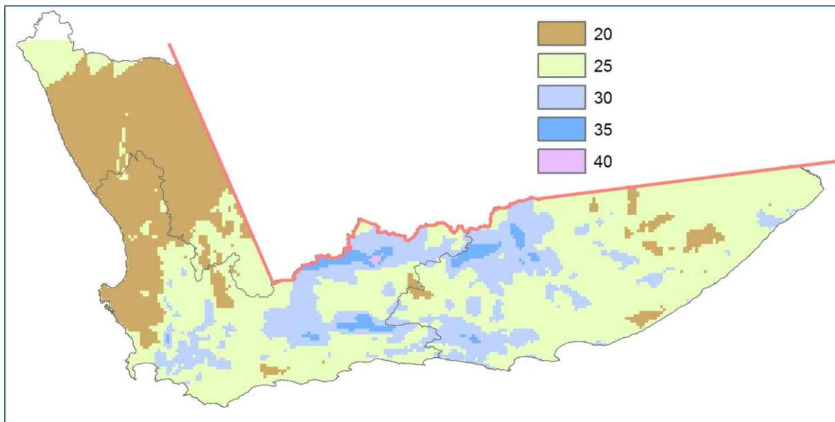
Figure 6. 1:50 Year 10 min wind speed (m/s) for the WASA domain, derived from model and measured data combined.
