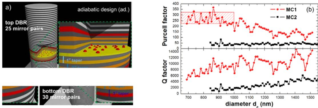
**Figure 1:** Schematic sketch of the adiabatic AlAs/GaAs micropillar cavity design with 25/30 mirror pairs in the top/bottom DBR. A zoom in picture in the cavity taper region is added (a). Comparative measurements of Q were performed between MC1 and MC2 (b; bottom). Purcell factors for MC1 between 225 and 325 can be expected for micropillars with  $d_c$  between 0.70  $\mu\text{m}$  and 1.00  $\mu\text{m}$  (indicated by the shaded box) (b; top)
