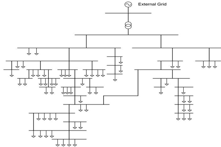
**Figure 2 Bornholm 400 V Grid Model in PowerFactory**
