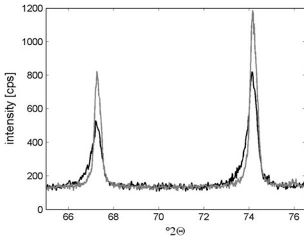
Fig. 3—Example of line profiles measured after the second (41  $\mu\text{m}$ , gray) and the fifth (144  $\mu\text{m}$ , black) removal of the steamside oxide on X20CrMoV12-1. The intensity maxima correspond to the magnetite phase.
