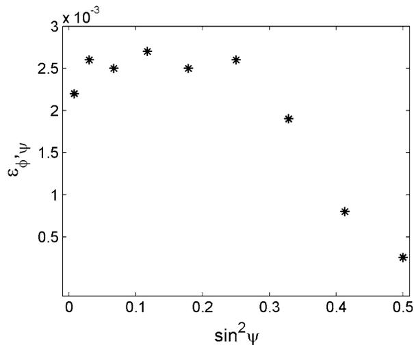
Fig. 9—Typical lattice strain distribution measured on the steamside, *i.e.*, the inner side, of ring samples of the fine-grained austenitic steel tube (example shown: sample TP-FG,  $\phi = 0$ , hematite).
