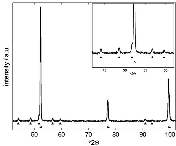
Fig. 5—X-ray diffractogram measured on the concave (steamside) surface of X20CrMoV12-1 after removal of approximately 260  $\mu\text{m}$  from the original surface; the magnification of a selected range is shown in the upper right corner. The theoretical positions of Bragg angles corresponding to  $\text{Cr}_{23}\text{C}_6$  carbides (closed triangles) and  $\alpha$ -iron (open triangles) are marked.
