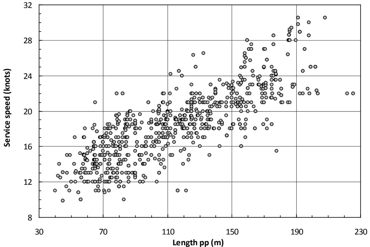
Fig. 10 Service speed of Ro-Ro passenger ships (ShipPax 2011).
