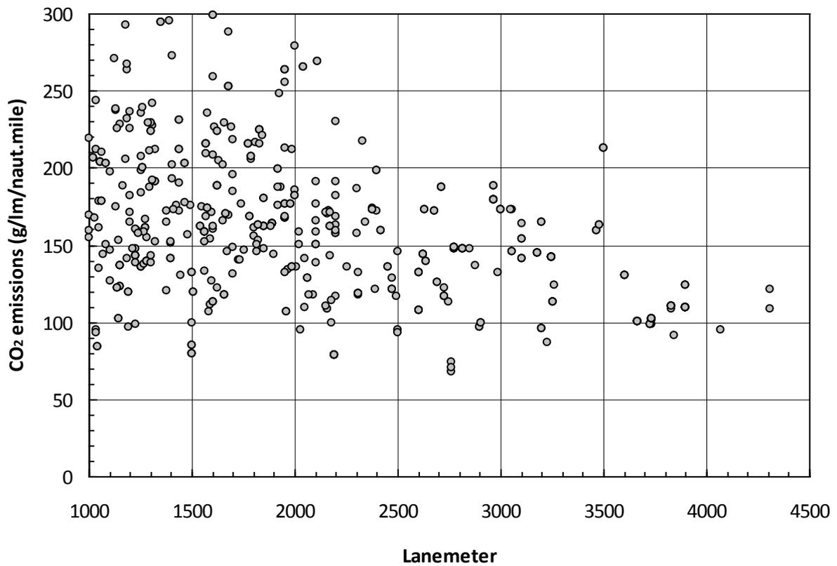
Fig. 12 CO<sub>2</sub> emissions per lane metre per nautical mile of Ro-Ro cargo ships (ShipPax 2011).
