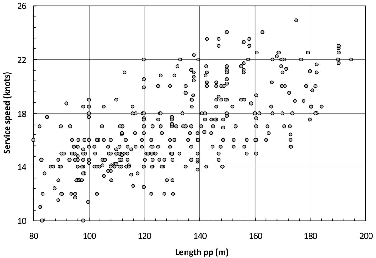
Fig. 11 Service speed of Ro-Ro cargo ships (ShipPax 2011).
