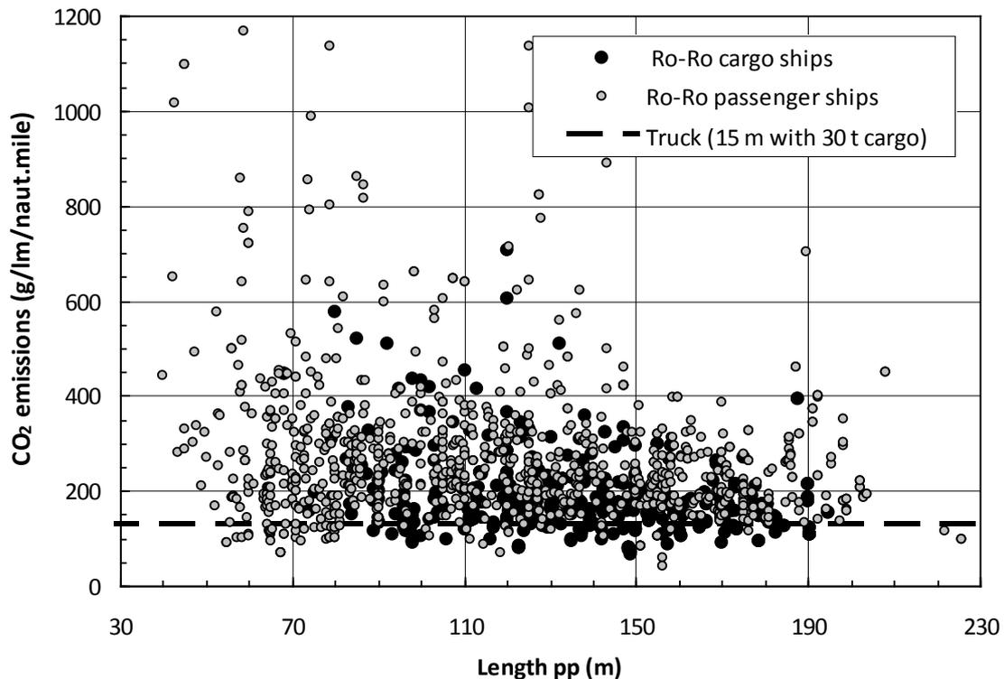
Fig. 13 CO<sub>2</sub> emissions per lane metre per nautical mile of Ro-Ro ships versus trucks.
