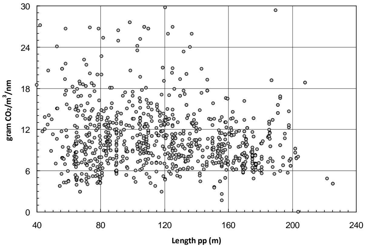
Fig. 9 CO<sub>2</sub> emissions per m<sup>3</sup> per nautical mile of Ro-Ro passenger ships (ShipPax 2011).
