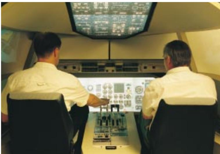
simulated by means of touch-sensitive display screens. A cockpit simulator of this design makes it possible to accommodate a variety of aircraft types and models. The prototype developed in the project simulates the cockpit of a Saab 340 twin-propeller commuter plane. Its touch-screen panels are mounted in a cockpit mock-up with added paper-tiger parts and demo objects for those parts of the cockpit equipment, which are not simulated with touch screens.
