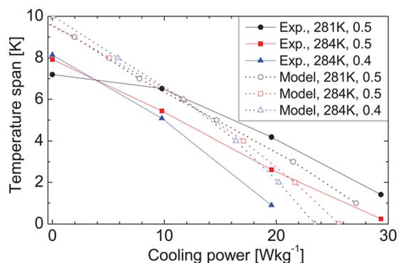
FIG. 3. (Color online) Cooling curves obtained at a mass flow rate of  $2.63 \text{ gs}^{-1}$  for both experiments and model predictions. Each curve is indexed by the hot end temperature and the utilization. The lines are guides to the eye.
