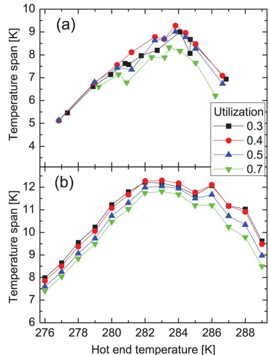
FIG. 2. (Color online) Temperature spans obtained at a mass flow rate of  $1.32 \text{ gs}^{-1}$ . (a) gives experimental results and (b) gives the predictions of the numerical model. The lines are guides to the eye.
