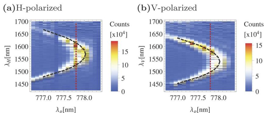
**Figure 2 | Intensity plots of the measured single photon spectra for (a) horizontal and (b) vertical polarized SPDC-output from the chip, versus the wavelength of the pump laser.** The dashed lines are theoretical predictions indicating where the TIR modes are perfectly phase matched to a single frequency pump. The CW pump wavelength used for the polarization entanglement measurements is marked with the red dotted lines<sup>29</sup>.
