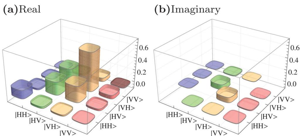
**Figure 4 | Reconstructed polarization state generated by the BRW.** The panels show real (a) and imaginary (b) parts of the state. The resulting density matrix entanglement measure, concurrence, equals 0.52. The fidelity with the Bell state  $(|HV\rangle + |VH\rangle)/\sqrt{2}$  state is 0.83 and the purity is 0.64.
