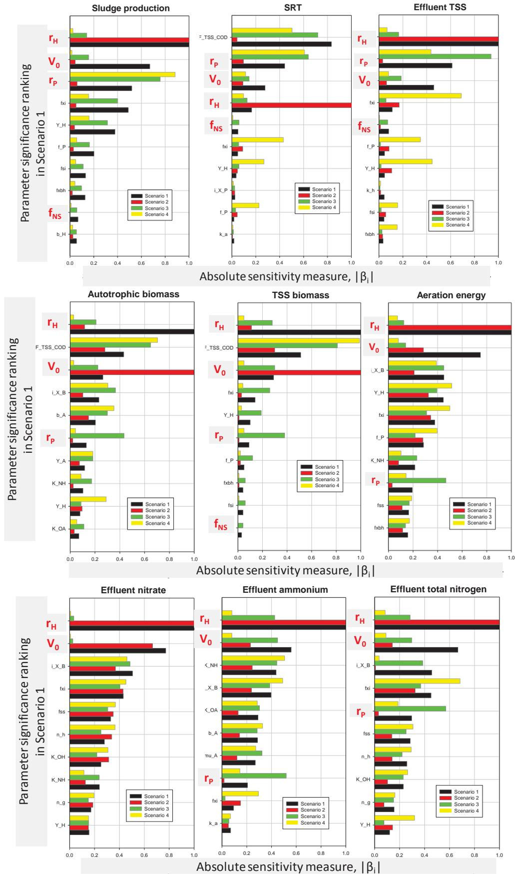
Figure 2 | Values of the relative sensitivity measure ( $\beta_i$ ) plotted as a function of the first ten model parameters ranked in Scenario 1 for the nine plant performance criteria (PPC). Additionally, simulation
