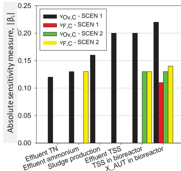
**Figure 5** | Values of the absolute sensitivity measure ( $\beta_i$ ), obtained for two parameters of the hydraulic sub-model of the Plósz-model (Scenarios 1-2), plotted as a function of the performance criteria, in which,  $\beta_i > 1$ .
