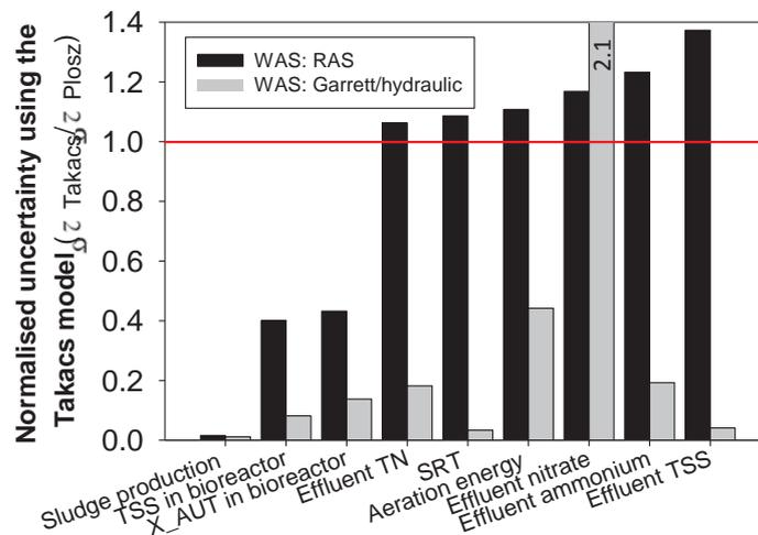
**Figure 1** | Values of the variance for each PCC obtained using the first-order Takács-model in the BSM1, normalised to data obtained with the convection-dispersion SST model. The two different simulation model structures include sludge wastage via the last aerobic tank (Garrett-method) or via the RAS.
