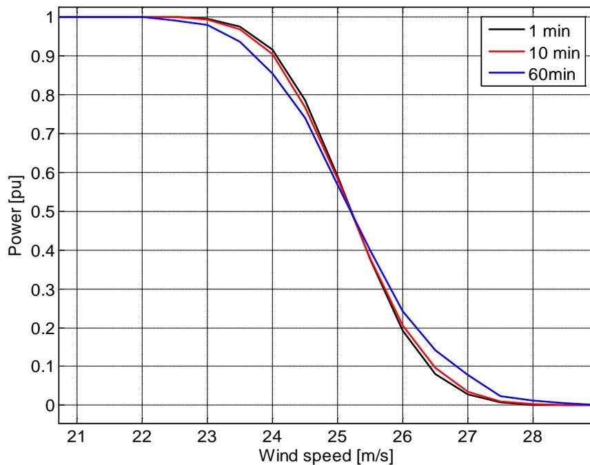
**Figure 13** Detail of aggregated wind power curve
