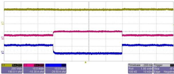
Figure 20. Transient response with respect to the input current disturbances under conditions:  $V_{g1}=50V$ ,  $V_{g2}=30V$ . Ch1: output voltage  $v_o$  [200 V/div], Ch2:  $i_{g1}$  [10 A/div], Ch3:  $i_{g1}$  [10 A/div]. (Time base: 1s/div)
