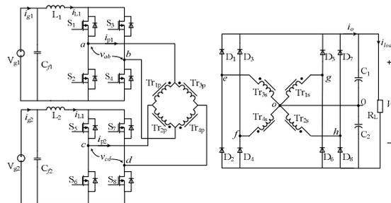
Figure 2. The proposed dual-input isolated full-bridge boost converter.
