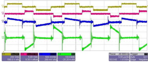
Figure 18. Experimental waveforms of the transformer primary side voltages and currents, Ch1:  $v_{ab}$  [200 V/div], Ch2:  $v_{ab}$  [250 V/div], Ch3:  $i_{p1}$  [10 A/div], Ch4:  $i_{p2}$  [10 A/div]. (Time base: 5  $\mu$ S/div)
