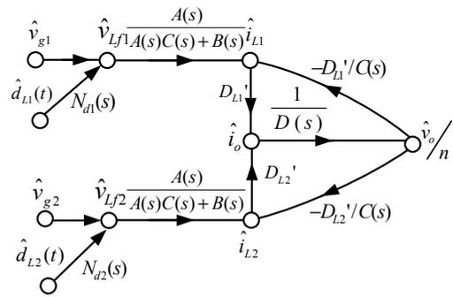
Figure 12. The simplified and reshaped small-signal (SS) model.
