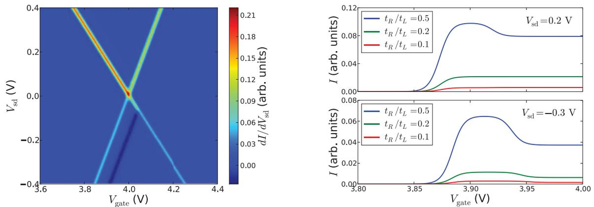
FIG. 6. (Color online)  $I$ - $V$  characteristics for the asymmetric setup where the distance to the right electrode is twice the distance to the left electrode and with coupling in the para configuration. Left: Stability diagram for  $\theta = \pi/12 \sim 0.26$ ,  $k_B T = 5$  meV, and  $t_L = 10t_R$ . Right: Absolute value of the current vs gate voltage for different values of the tunnel coupling ratio  $t_R/t_L$  at positive and negative bias voltage.
