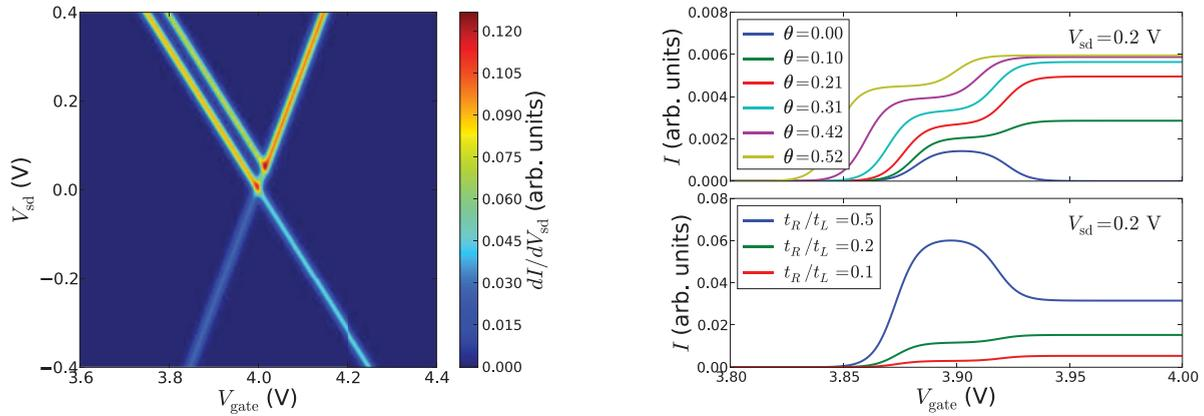
FIG. 7. (Color online)  $I$ - $V$  characteristics for the asymmetric setup with coupling in the meta configuration. Left: Stability diagram for the same set of parameters as in Fig. 6. Right: Absolute value of the current vs gate voltage for different values of the rotation angle  $\theta$  at  $t_L = 10t_R$  (upper) and the tunnel coupling ratio  $t_R/t_L$  at  $\theta = \pi/12$  (lower). Note the collapse of the current for  $\theta = 0$  in the upper plot.
