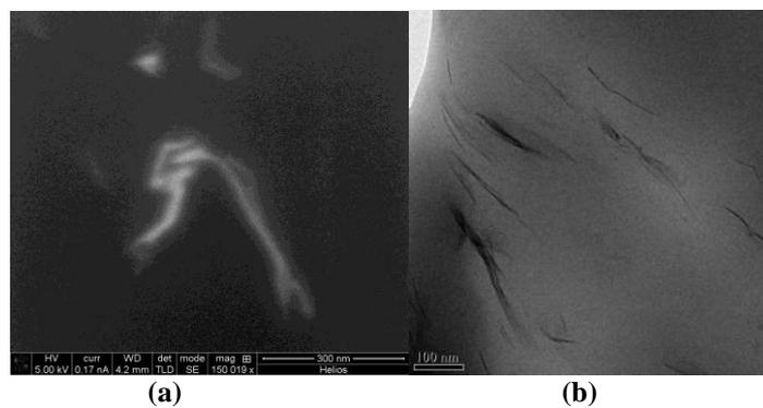
**Figure 3.** High resolution SEM (a) and TEM (b) micrographs recorded at comparable magnifications of the clay/PP nanocomposite studied in this work.
