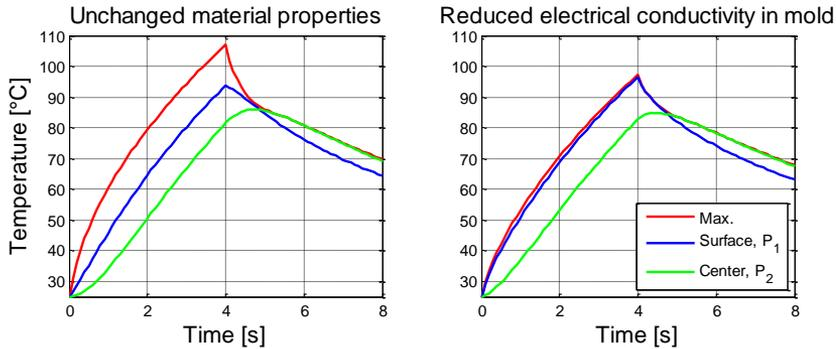
Fig.8. Comparison of the temperature at the surface above the inductor ( $P_1$ ), center of the mold ( $P_2$ ), and the maximum temperature, during four seconds of heating and four seconds of cooling, without (left) (unfavorable) and with (right) (favorable) a ten time reduction in the electrical conductivity of the mold.
