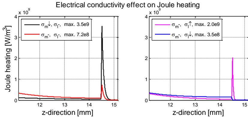
Fig.6. Distribution of the Joule heat in the z-direction above the inductor for different electrical conductivities,  $\sigma$ , in the mold (denoted with m) and the layer (denoted with l). Downward pointing arrow means a ten times lower conductivity, and upward pointing arrow means a ten times higher. Having a low electrical conductivity in the mold is favorable.
