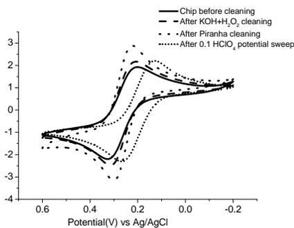
Figure 1 Comparison study of CV scans obtained on the gold electrodes before cleaning, and after cleaning with KOH+H<sub>2</sub>O<sub>2</sub>, Piranha, and potential sweep in HClO<sub>4</sub>.
