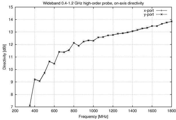
Figure 6. The measured on-axis directivity versus frequency of the quad-ridge horn.
