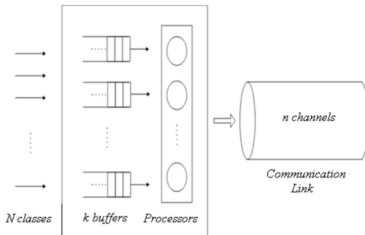
Fig. 1: Resource allocation in a network communication link [3].
