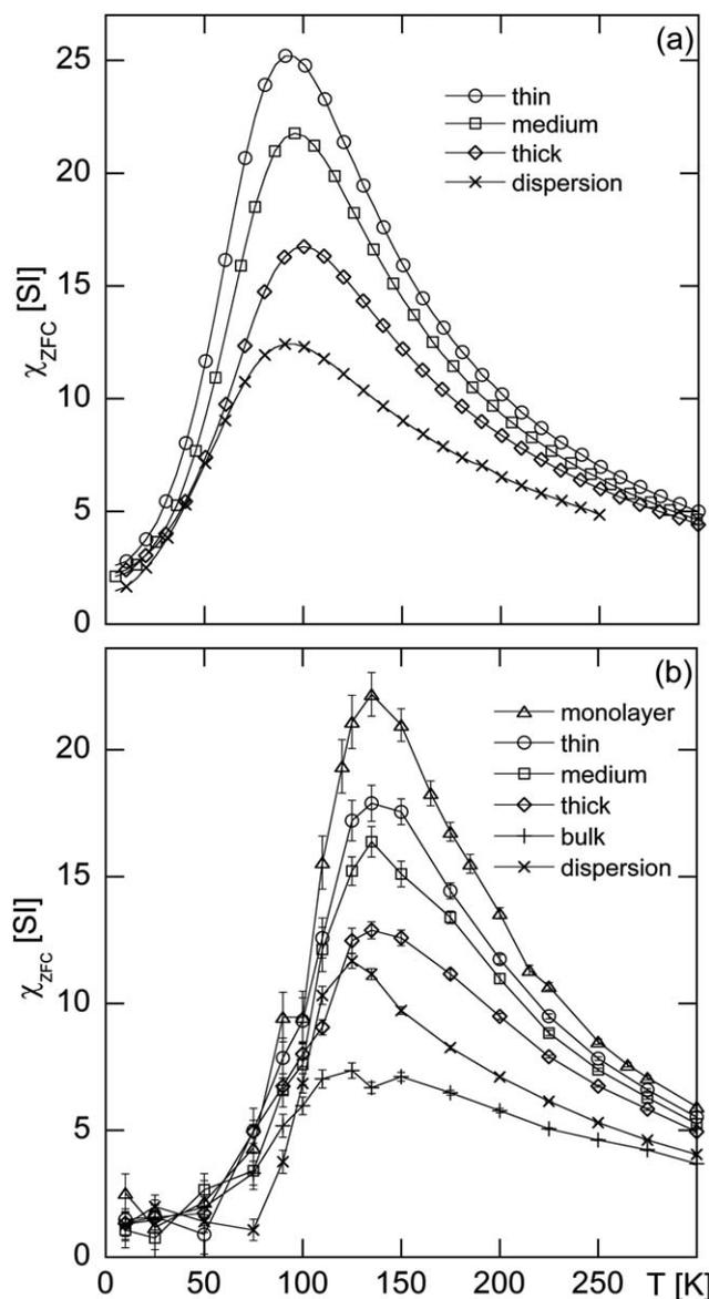
**Fig. 4** ZFC in-plane susceptibility vs. temperature curves at intermediate field ( $H = 1.6 \text{ kA m}^{-1}$ ). The solid lines are guides to the eye. (a) Experimental curves for the arrays and the dispersion. (b) Curves obtained from the MC simulations. Each point is the average of 25 to 325 independent simulations, with a standard error shown by the error bars.
