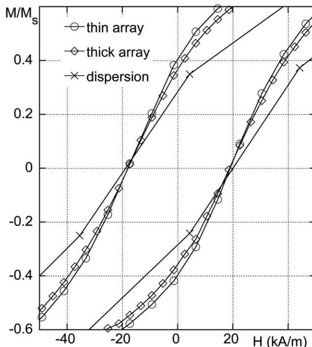
**Fig. 2** Normalized magnetization  $M/M_s$  versus the applied field  $H$  (hysteresis loops) for the thin (O) and thick ( $\diamond$ ) arrays and for the dispersion (x) at 10 K. The data have been corrected for an exchange bias effect,<sup>44</sup> and the full hysteresis loops are available in the ESI.† The lines are guides to the eye.
