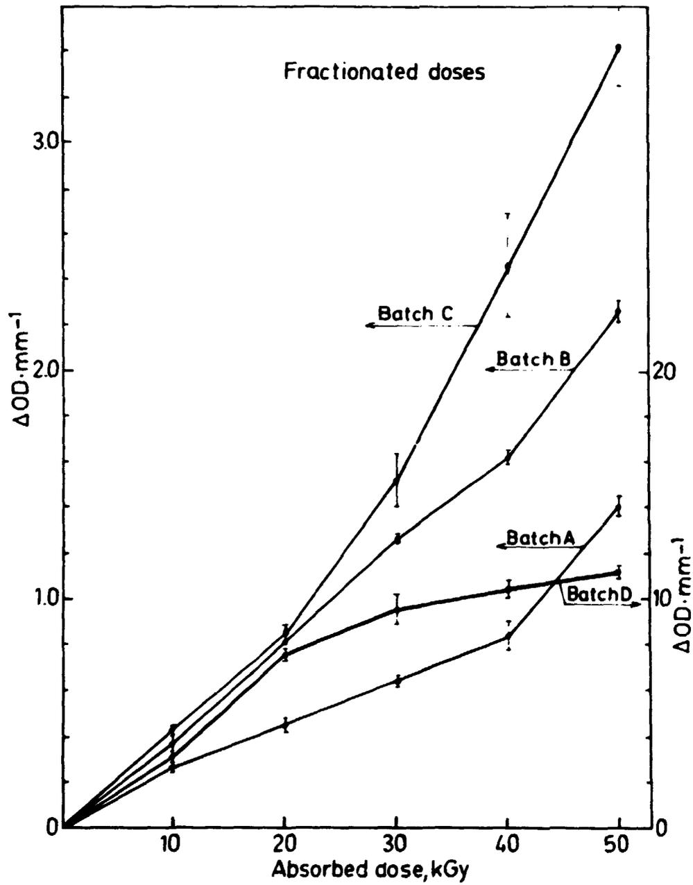
Fig. 2b. Change in optical density divided by thickness ( $\Delta OD \cdot mm^{-1}$ ) versus dose for the 4 PVC-films. The dose in fractions of 10 kGy.
