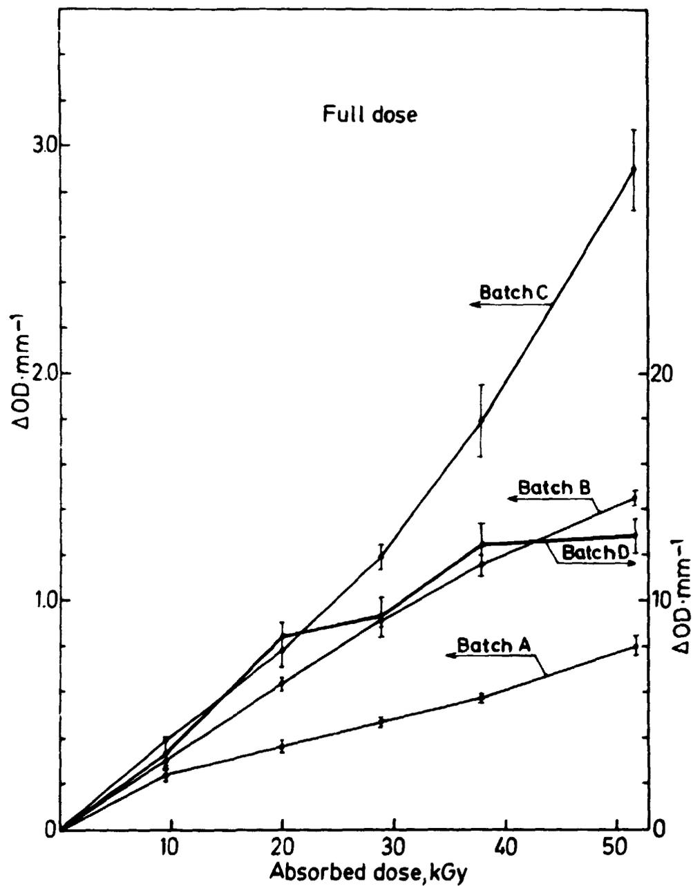
Fig. 2a. Change in optical density divided by thickness ( $\Delta OD \cdot mm^{-1}$ ) versus dose for the 4 PVC-films. The dose in full doses.
