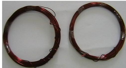
Fig. 13. Two ring-shaped armature windings.
