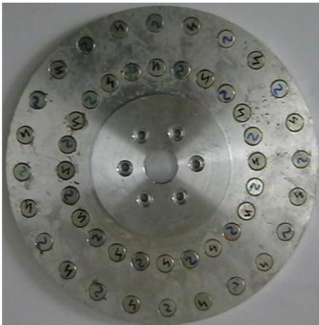
Fig. 11. Rotor Disk with circular flat shaped PMs.
