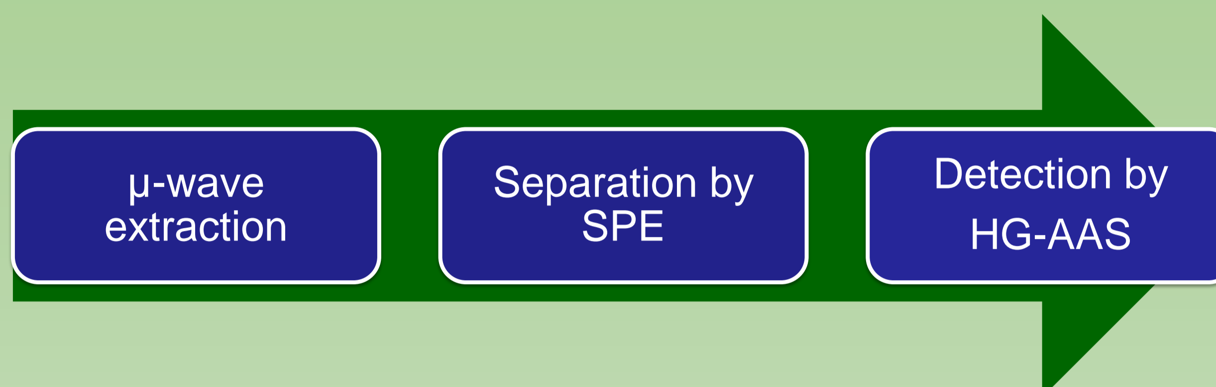
FIGURE 1. Principle of the MAE-SPE-HG-AAS approach for selective speciation analysis of inorganic arsenic.
