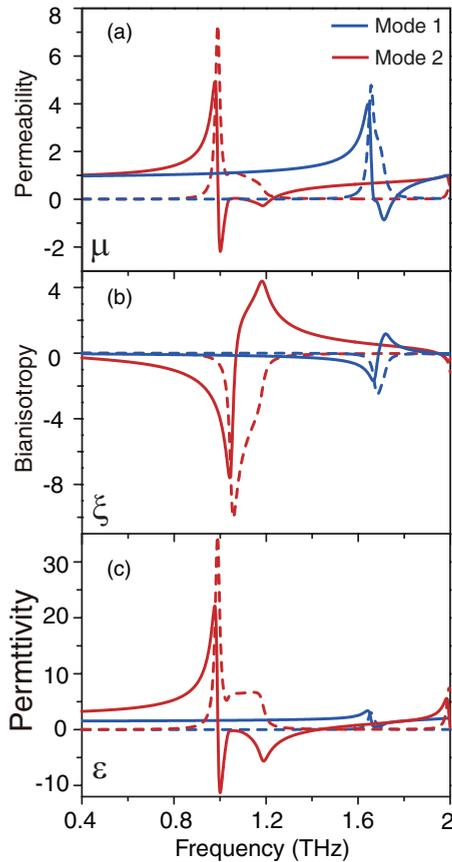
FIG. 3. (Color online) Retrieved constitutive parameters of (a) permeability  $\mu$ , (b) bianisotropy parameter  $\xi$ , and (c) permittivity  $\epsilon$ , from full wave electromagnetic simulations of the 3D DSRRs. The blue lines represent the parameters at mode 1 (i.e., no photoexcitation). The red lines represent the parameters at mode 2 assuming the bottom gap is shorted by replacing the silicon by copper. Solid lines are real parts and dashed lines are imaginary parts.
