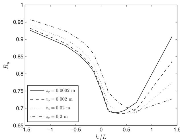
**Figure 3.** The wind-speed reduction  $R_u$  of the extended IWFBL model of Frandsen for a range of dimensionless atmospheric stabilities  $h/L$ , a number of surface roughness values  $z_o$  (see legend) and a fixed dimensionless turbine–turbine separation  $s = 7$ . The model is evaluated with  $C_t = 0.88$ ,  $h = 70$  m,  $u_{h\text{free}} = 10$  m s<sup>-1</sup> and latitude of 55.5°.
