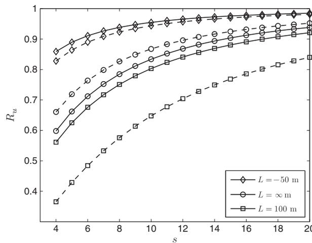
**Figure 4.** A comparison between the wind-speed reduction  $R_u$  of the extended IWFBL model by Frandsen (solid lines) and the model by Emeis<sup>20</sup> (dashed lines) for different atmospheric stabilities (see legend) and dimensionless turbine–turbine distances  $s$ . The models are evaluated with  $C_t = 0.88$ ,  $h = 70$  m,  $u_{h\text{free}} = 10$  m s<sup>-1</sup>,  $z_o = 0.0002$  m and latitude of 55.5°.
