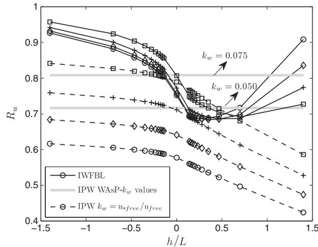
**Figure 9.** As in Figure 7 but for a range of dimensionless atmospheric stability conditions  $h/L$  and a constant dimensionless turbine–turbine separation  $s = 7$ . The models are evaluated with  $h = 70$  m,  $D_r = 80$  m,  $u_{hfree} = 10$  m s $^{-1}$  and latitude of 55.5°.
