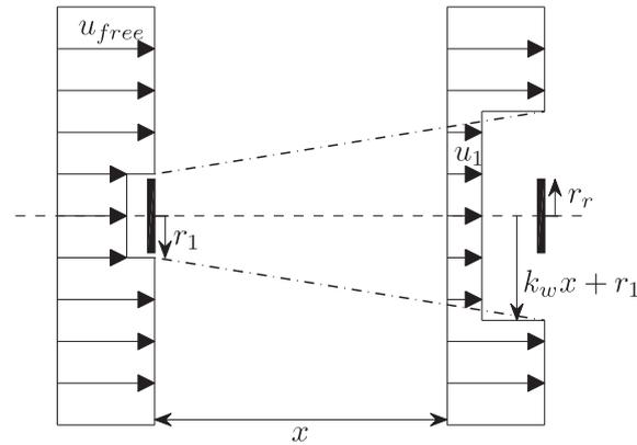
**Figure 6.** Momentum wake model concept by Jensen.<sup>25</sup> The wind speed immediately before a wake-affected turbine  $u_1$  is estimated as a function of the distance to the upstream turbine  $x$  with rotor radius  $r_r$ , the free wind speed  $u_{free}$ , and the thrust coefficient and the wake-decay coefficient  $k_w$ .
