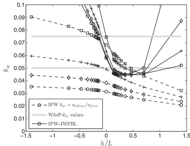
**Figure 10.** As in Figure 8 but for a range of dimensionless atmospheric stability conditions  $h/L$  and a constant dimensionless turbine–turbine separation  $s = 7$ . The models are evaluated with  $h = 70$  m,  $D_r = 80$  m,  $u_{hfree} = 10$  m s $^{-1}$  and latitude of 55.5°.
