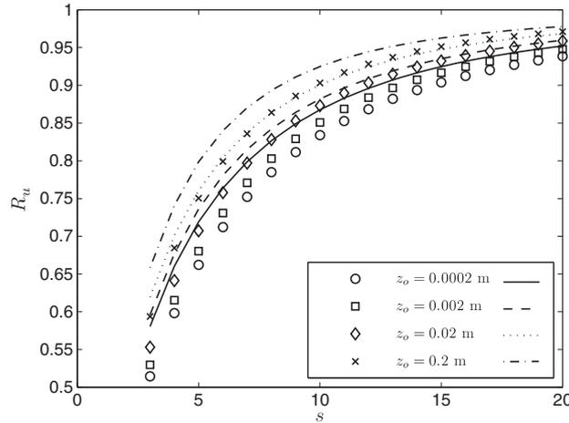
**Figure 2.** Wind speed reduction  $R_u$  comparison between the IWFBL models of Frandsen<sup>9</sup> (in markers) and E&F<sup>15</sup> (in lines) for different dimensionless turbine to turbine separations  $s$  and surface roughness values  $z_o$  (see legend). The models are evaluated with  $C_t = 0.88$ ,  $h = 70$  m,  $u_{\text{free}} = 10$  m s<sup>-1</sup>,  $z_o = 0.0002$  m,  $A_* = 4.53$  and latitude of 55.5°.
