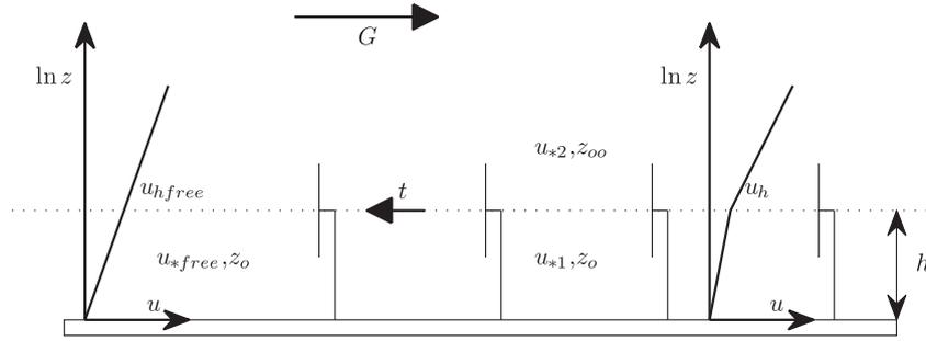
**Figure 1.** The infinite wind-farm boundary-layer model concept of Frandsen.<sup>9</sup> Upstream of the wind farm (free flow), there is one layer with the undisturbed stress scale and background roughness ( $u_{*free}, z_o$ ), and within the wind farm, two layers are assumed to meet at hub height  $h$ : the lowest with the background roughness and a low-stress-scale  $u_{*1}$ , and the highest with the effective wind-farm roughness  $z_{oo}$  and a high-stress-scale  $u_{*2}$ .
