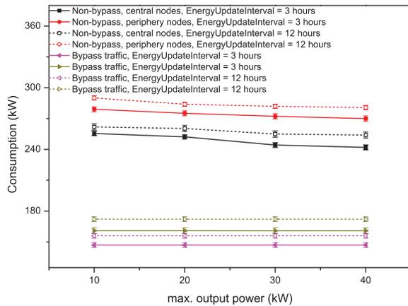
Fig. 5. Consumption of central nodes vs. periphery nodes.
