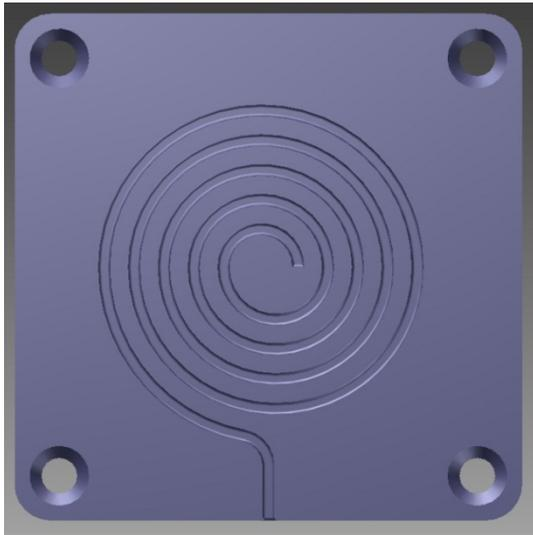
Figure 2: CAD model of the spiral mold insert
