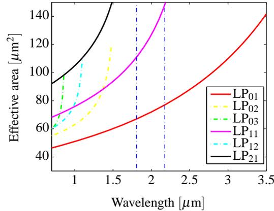
Fig. 5. Effective areas (inverse overlap integrals  $1/f_{01,xy}$ , where  $LP_{xy}$  is given by legend) for Raman scattering into 6 modes from the  $LP_{01}$  mode. The blue dashed lines are the pump wavelengths used for the upconversion experiments.
