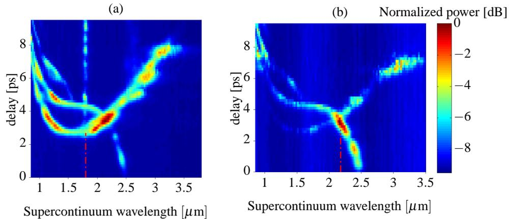
Fig. 3. Spectrograms resulting from the crosscorrelation are obtained by changing crystal phase matching angle. The fiber is pumped with a central wavelength of (a)  $1.8 \mu\text{m}$  and (b)  $2.2 \mu\text{m}$ , respectively (red dashed lines). The intensities are plotted on a dB scale. The pulse energy including coupling losses is in both cases approximately 30 nJ
