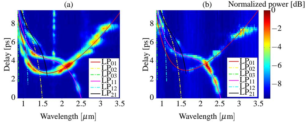
Fig. 4. The spectrograms from Fig. 3 plotted with arrival time calculations for the LP<sub>01</sub>, LP<sub>11</sub> and LP<sub>21</sub> modes. The spectrograms are in good agreement with the calculated arrival times. (a) Pump at 1.8 μm (b) Pump at 2.2 μm. The intensities are plotted on a dB scale.
