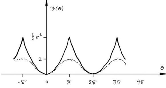
Fig. 2: Periodic parametric potential (18) originating from the potential in (2). The dashed curve corresponds to the Wilson analogue [14] of the Manton action and is not considered in the present work.
