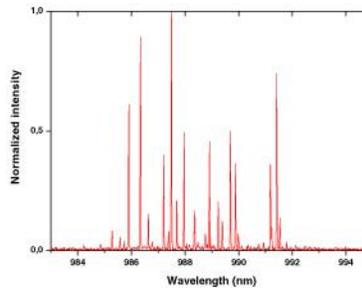
Fig. 5. The free running spectrum of the laser bar at I= 30A and the laser operating at 20°C.
