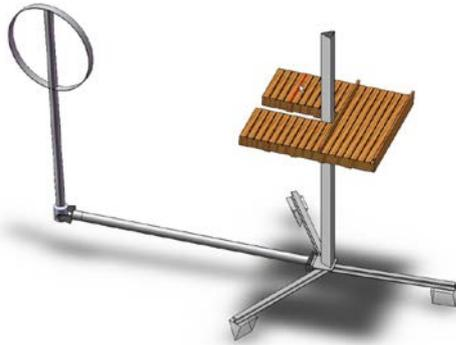
Figure 1 Principle test setup of 1kW DeepWind demonstrator wind turbine
