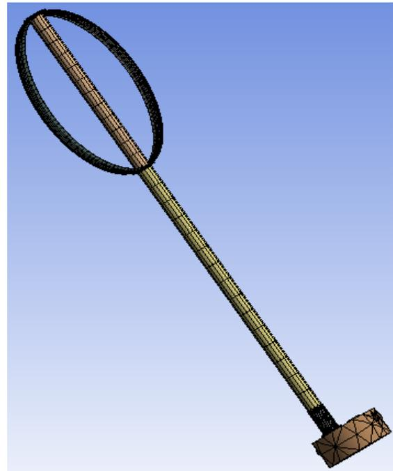
Figure 4 Model of 3<sup>rd</sup> configuration (tube, blade and generator) for modal testing
