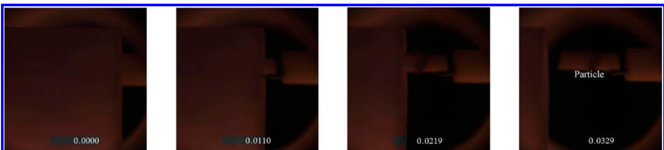
Figure 3. Removing the protection tube from the left to the right: at t = 0.000 s, the cylindrical particle is entirely covered by the tube; at t = 0.0329 s, the cylindrical particle is entirely exposed to the hot flow in the reactor.
