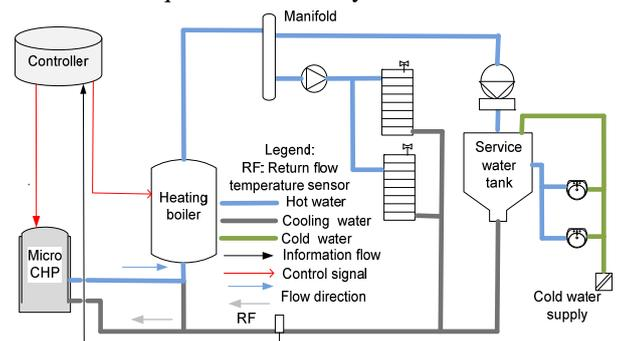
Fig. 2 Physical layout 1 of the heating system
