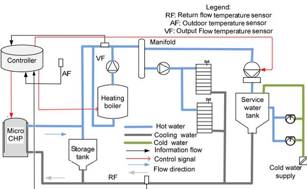
Fig. 4 Physical layout 3 of the heating system
