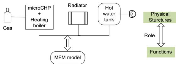
Fig. 1 Main scheme of the heating system
