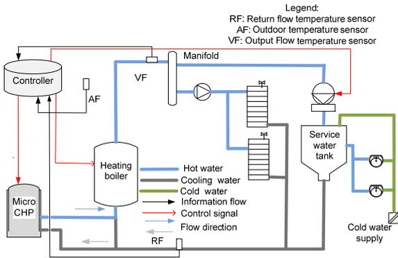
Fig. 3 Physical layout 2 of the heating system
