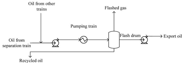
Figure 6: Flow sheet of the export pumping train
