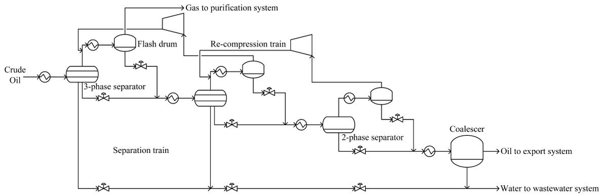
Figure 3: Flow sheet of the separation and gas re-compression trains
