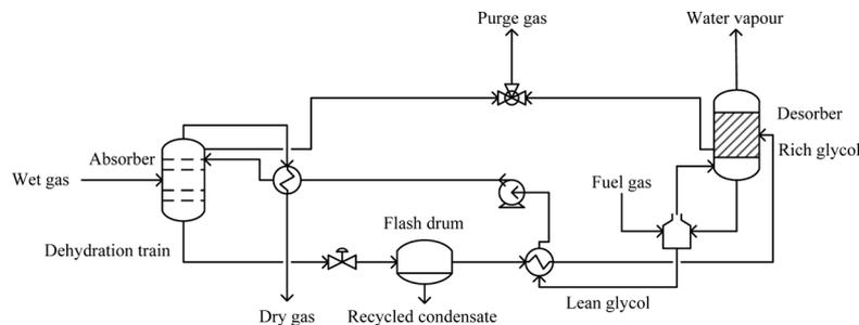
Figure 4: Flow sheet of the glycol dehydration unit
