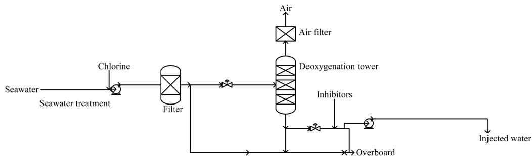
Figure 7: Flow sheet of the seawater injection system
