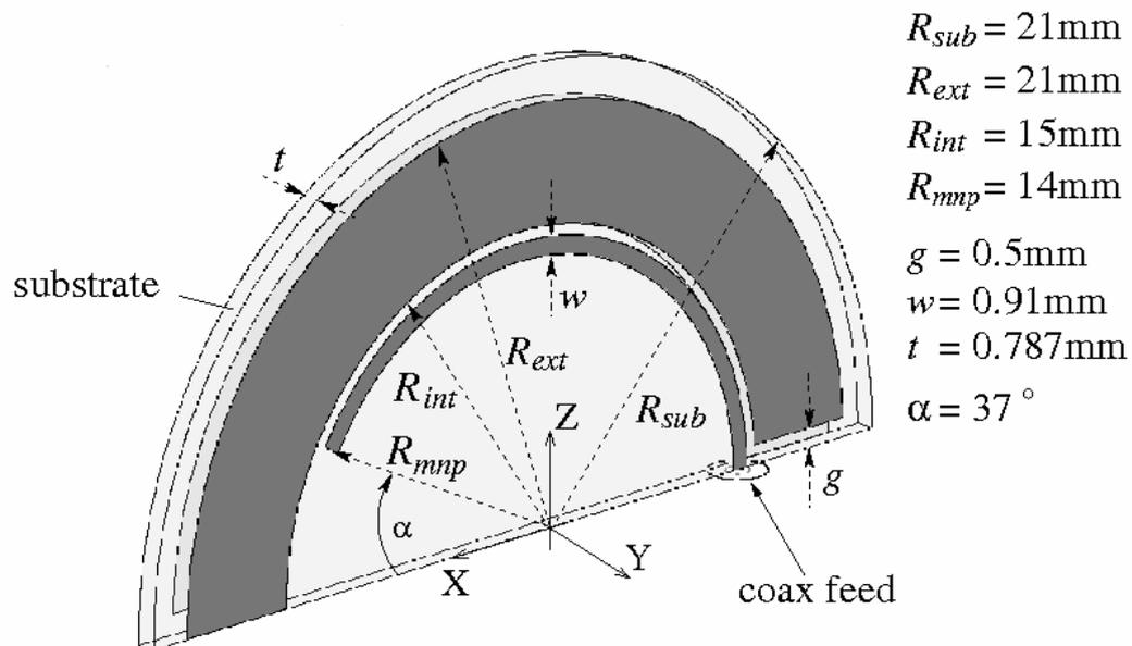
Fig. 1 Geometry of the SRR-based electrically small antenna
