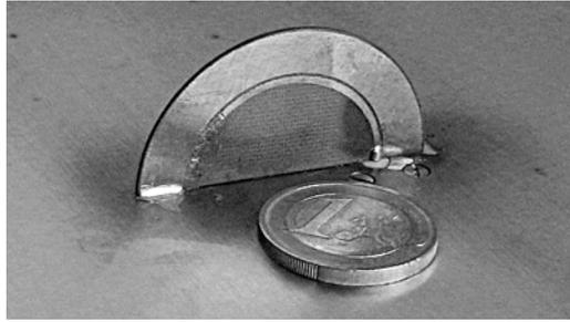
Fig. 3 Manufactured prototype of the SRR-based electrically small antenna
