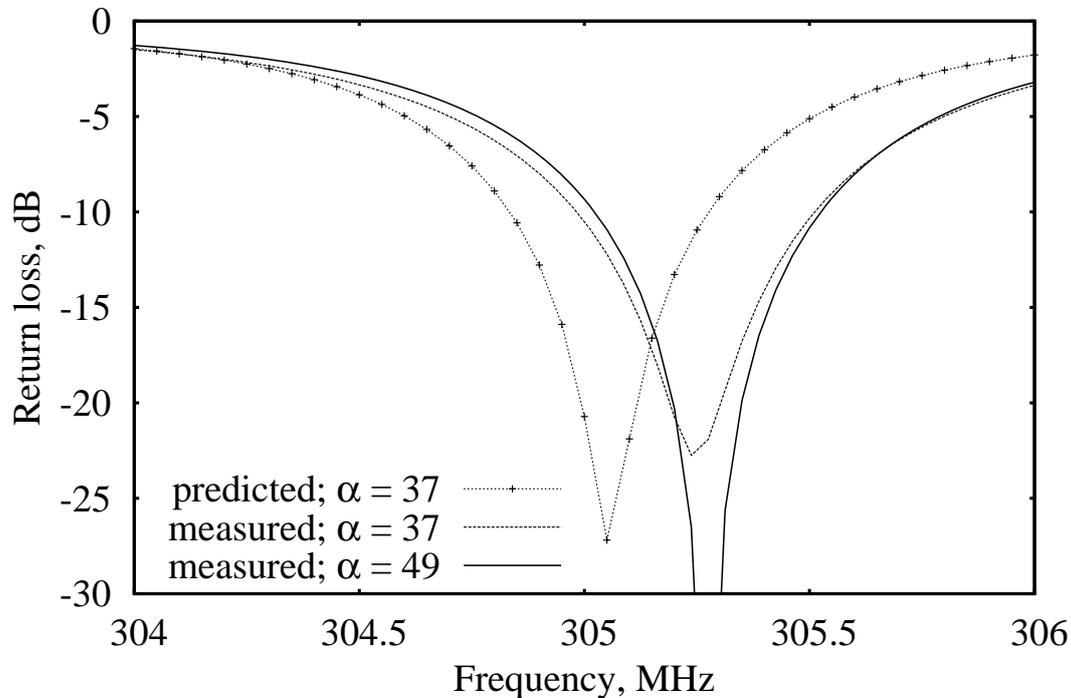
Fig. 2 Predicted and measured return loss
