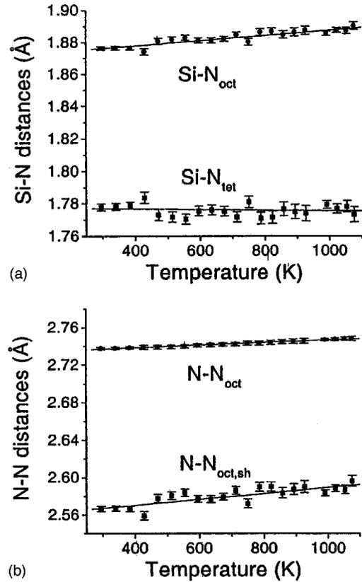
FIG. 2. Temperature dependences of bond lengths for the tetrahedral and octahedral Si-N pairs (a) and N-N pairs (b) obtained from the Rietveld structural refinements for the  $c\text{-Si}_3\text{N}_4$  phase.
