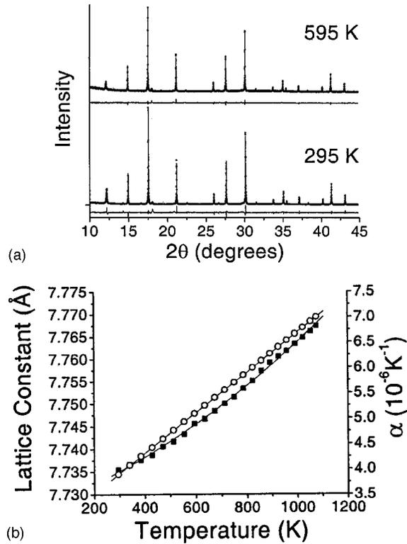
FIG. 1. (a) Rietveld structural refinement profiles of two x-ray powder-diffraction data recorded at 295 and 595 K for the cubic spinel  $\text{Si}_3\text{N}_4$  phase. (b) The lattice parameter (solid squares) and the linear thermal expansion coefficient (open circles) of the  $c\text{-Si}_3\text{N}_4$  phase together with fitted curves.
