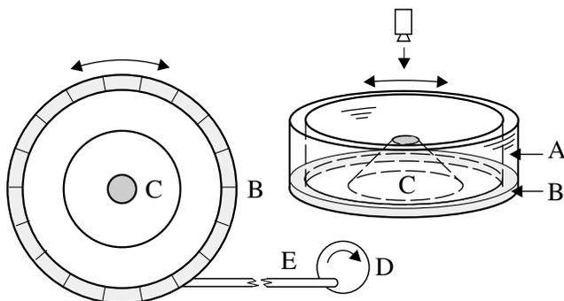
FIG. 2. A sketch of the experimental setup seen from above (left) and from the side (right). The length of the arm  $E$  and the width of the channel are not to scale. See text.
