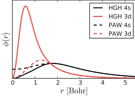
FIG. 1. (Color online) The pseudovalence states of iron calculated with PAW and the norm-conserving HGH pseudopotentials. Both methods produce smooth wave functions for the delocalized 4s state but the lack of norm conservation allows the short-ranged 3d state in PAW to be accurately sampled on a much coarser grid.
