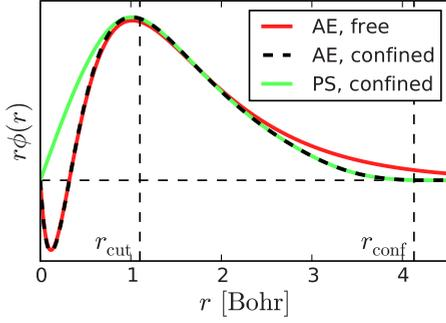
FIG. 2. (Color online) Basis function generation for the nitrogen  $2s$  state: the all-electron orbital of the free atom, the confined all-electron orbital, and the corresponding pseudowave function after applying the inverse PAW transformation. The augmentation sphere and basis function cutoffs are indicated.
