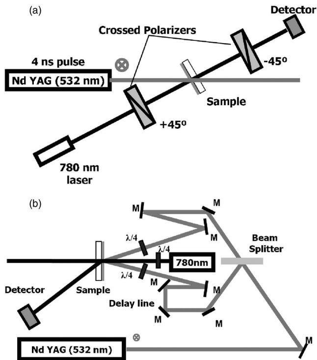
FIG. 2. Experimental setup for (a) photoinduced anisotropy measurements and (b) holographic polarization gratings recording and diffraction efficiency measurements.
