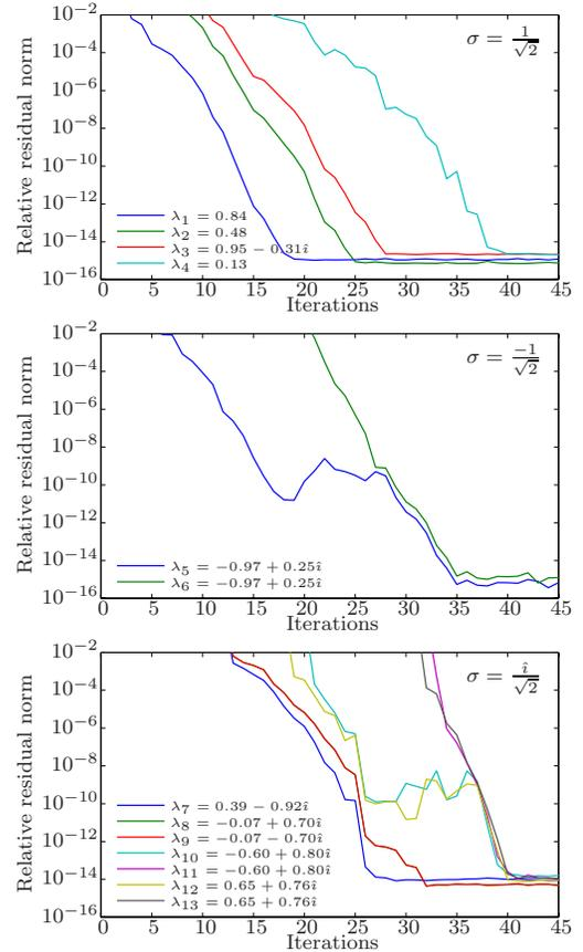
FIG. 4. (Color online) Convergence behavior of the Krylov algorithm for the Al(100) electrode at  $E = 3$  eV. The figures show the residual norm as a function of iterations for Ritz pairs that satisfy  $0.1 \leq |\lambda| \leq 1 + \epsilon$ , in the case of shift-and-invert transformations to  $\pm 1/\sqrt{2}$  and  $\hat{i}/\sqrt{2}$ , respectively.
