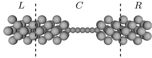
FIG. 5. Schematic illustration of the Al(100)-C7-Al(100) two-probe system.
