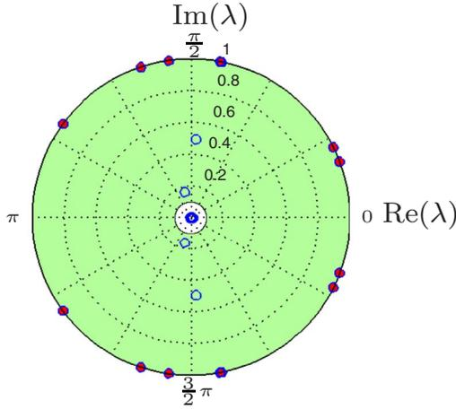
FIG. 2. (Color online) Positions of the 243 complex eigenvalues [blue (circles)] inside the unit disk for a Au(111) electrode with 27 atoms per unit cell at  $E = -2$  eV. The 21 eigenvalues corresponding to propagating modes [red (filled dots)] are located on the unit circle. The modes of most significance in transmission calculations are located within the green (shaded) area given by  $0.1 \leq |\lambda| \leq 1$ .
