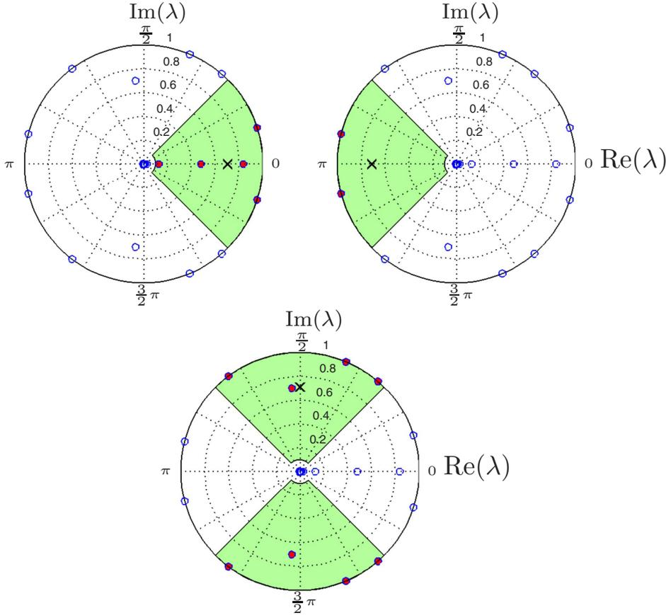
FIG. 3. (Color online) Illustration of the complex eigenvalues [blue (circles)] for the Al(100) electrode at  $E=3$  eV. The eigenvalues corresponding to the wanted right-going modes [red (filled dots)] can be separated according to their location within three distinct green (shaded) areas of the unit disk and determined efficiently using shift-and-invert spectral transformations to  $\pm 1/\sqrt{2}$  and  $i/\sqrt{2}$  (crosses).
