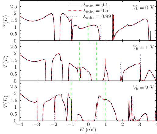
FIG. 6. (Color online) Transmission spectrum of the Al(100)-C7-Al(100) system for different bias voltages  $V_b$ . The self-energy matrices used in the  $T(E)$  calculations have been obtained at the  $\Gamma$  point by the proposed Krylov subspace method with parameter  $\lambda_{\min}$  at several settings: 0.1 [black (full) curve], 0.5 [red (dashed) curve], and 0.99 [blue (dotted) curve]. The bias windows are indicated by the vertical dashed lines.
