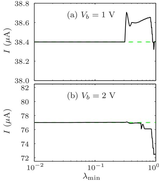
FIG. 7. (Color online) Current as a function of the parameter  $\lambda_{\min}$  used by the Krylov subspace method for the Al(100)-C7-Al(100) system with applied bias voltages  $V_b=$  (a) 1 and (b) 2 V. The correct currents obtained by conventional methods are  $I \approx 38.4$  and  $\approx 77.0$   $\mu\text{A}$ , respectively, indicated here by the green (dashed) lines.
