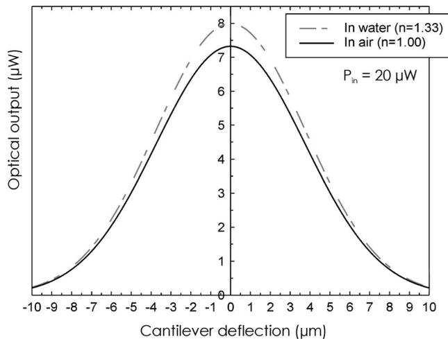
FIG. 3. When the medium between the cantilever waveguide and the output waveguide is water (or buffer solution) instead of air, the optical output is increased due to the reduced refractive index difference.
