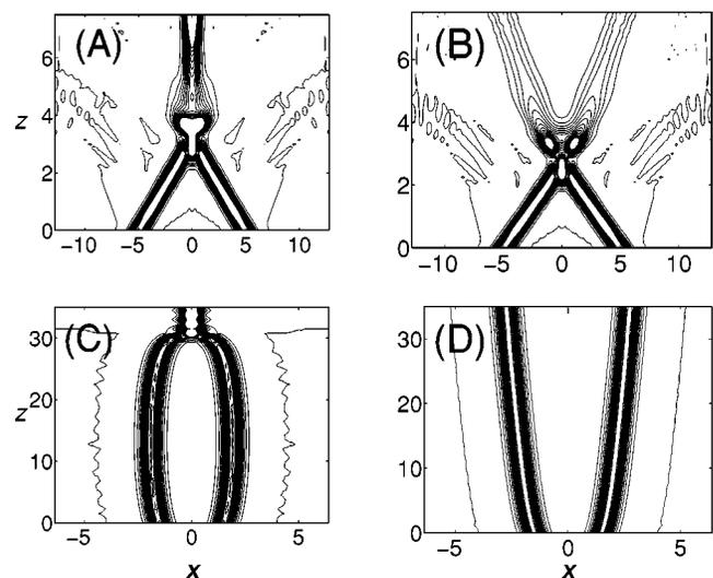
FIG. 1. (a),(b) Planar collision between two Gaussians,  $P=48.3$  and  $\beta=0$ . (c),(d) Outwards-launched exact solitons,  $P=122.4$  and  $\beta=5$ . The launch angles are  $\alpha_x=58^\circ$  (a),  $\alpha_x=62^\circ$  (b),  $\alpha_x=5.4^\circ$  (c), and  $\alpha_x=5.7^\circ$  (d).
