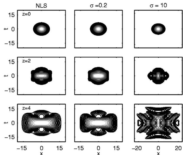
FIG. 4. Intensity profile of the FW,  $|E_1(x,t)|^2$ , at different propagation lengths for the modified X-wave case. Parameter values are  $A=5, B=3, d_1=-1$ , and  $d_2=+1$ . The NLS Eq. (3) solved for  $\sigma=0.2$  (left). Full equations solved for  $\sigma=0.2$  (center) and 10 (right). 15 contour lines from 0.001 logarithmically separated to the maximum intensity.
