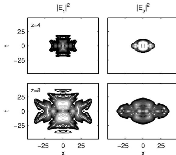
FIG. 6. Intensity profiles for the (left) FW,  $|E_1|^2$ , and (right) SH,  $|E_2|^2$ , at propagation lengths  $z=$  (top) 4 and (bottom) 8. Parameter values are  $A=5, B=3, d_1=-1, d_2=+1$ , and  $\sigma=10$ , i.e., strongly nonlocal. 15 contour lines from 0.005 logarithmically separated to the maximum intensity.
