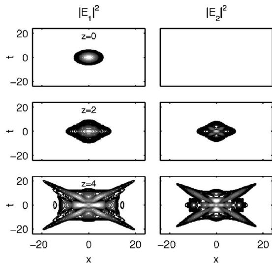
FIG. 9. Intensity profile of the strongly nonlocal X-wave case,  $\sigma = 10$ . The evolution of  $|E_1|^2$  (left) and  $|E_2|^2$  (right). Parameter values are  $A=5, B=3$ , and  $d_1 = d_2 = -1$ . 15 contour lines from 0.005 logarithmically separated to the maximum intensity.
