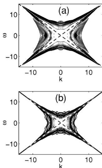
FIG. 10. Comparison between  $|\widetilde{E}_2|^2$  (a) and the nonlocal prediction  $(1/\beta)^2 |\widetilde{E}_1|^2 |\widetilde{R}|^2$  (b) at  $z=4$  with 25 logarithmically spaced contours between 0.0001 and 10. Parameter values are  $A=5, B=3$ , and  $d_1=d_2=-1$ .  $\sigma=10$ , i.e., strongly nonlocal. Dashed lines correspond to  $\sigma\omega = \pm\sqrt{1+\sigma^2k^2}$ .
