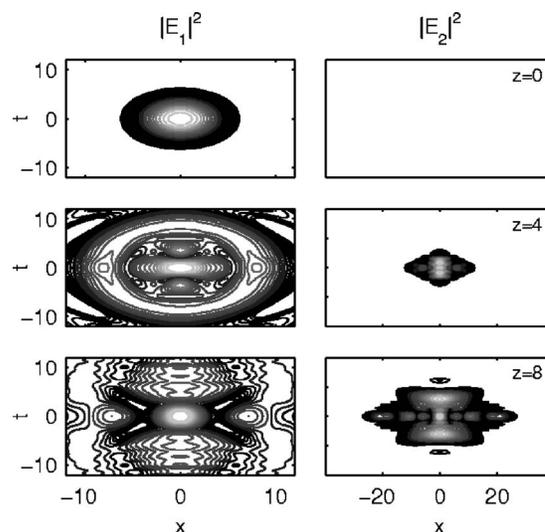
FIG. 11. FW and SH intensity profiles  $|E_1|^2$  (left) and  $|E_2|^2$  (right) at propagation lengths  $z=0, 4$ , and  $8$ . Parameter values are  $A=5, B=3$ , and  $d_1=-d_2=1$ . Strongly nonlocal case,  $\sigma=10$ . 25 contour lines from 0.005 logarithmically separated to the maximum intensity. The mesh size is 360 on a  $-50 < x, t < 50$  domain.
