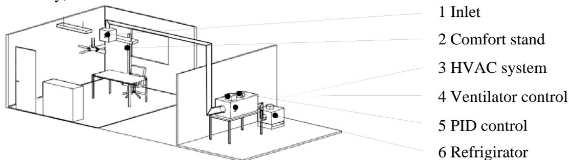
Figure 1. Schematic drawing of the climate room.
